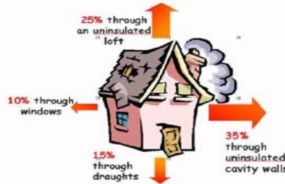
Typical Heat losses from un-insulation residential property.
